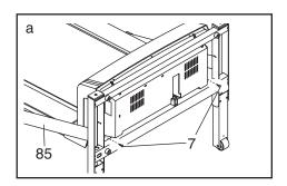
b. Raise the Upright (85) to the vertical position. Remove the three 3/4" Screws (7) from the Hood (33), and carefully pivot the Hood off.
